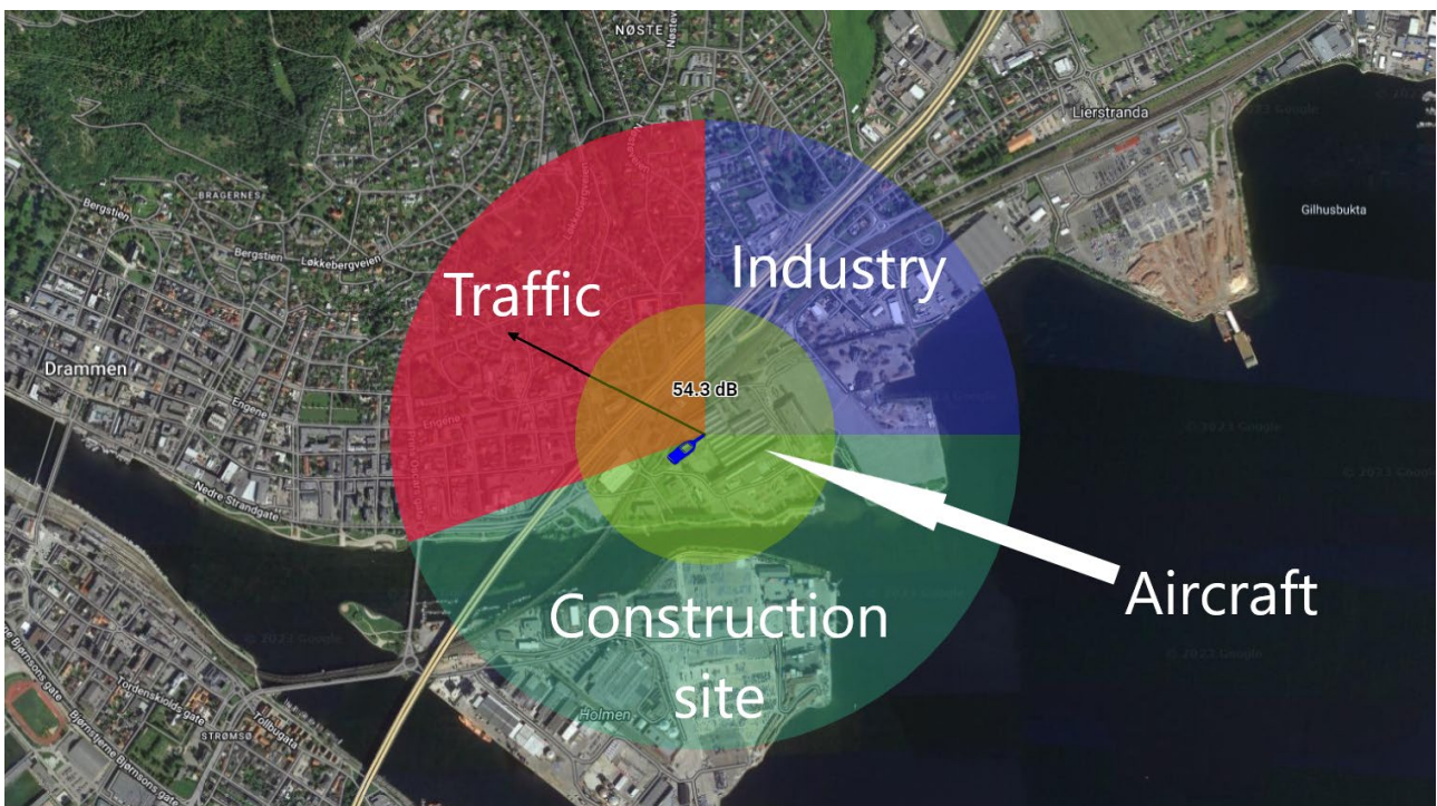
Figure 7 - Noise Compass sectors defined with NorCloud. Traffic, Industry and Construction site span different horizontal angles within vertical angles 0° to 60°. The sector Aircraft spans elevation angles 60° to 90°, for all horizontal angles.
