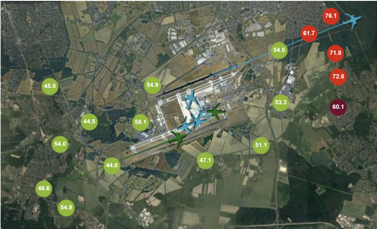
Figure 12 - Screenshot from the publicly accessible TRAVIS software. The figure shows the aircraft activity at Berlin Brandenburg airport in Germany, with associated L_{Aeq,1sec} levels measured by unattended noise monitoring stations. Noise Compass has been installed in some of these stations.
