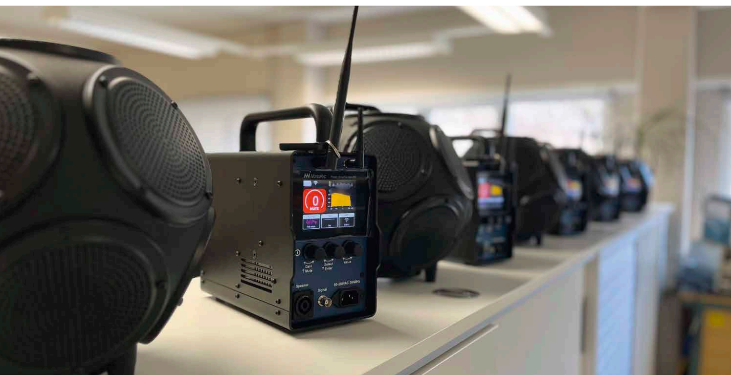
Nor283 dodecahedron loudspeakers and Nor282 power amplifiers ready for shipment.
