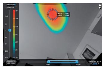
In addition to measurements in the living room subsequent measurements were also made in the two bedrooms. These measurements displayed the same result, the energy of the noise did not come from the walls, but were confined to the roof. All in all this was a very strong indication that the problem was piping located in separating floors between apartments.
