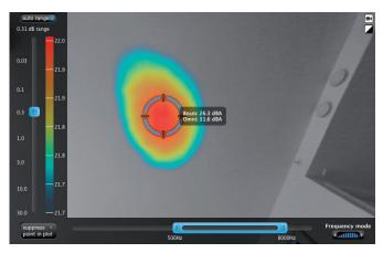
By using the virtual microphone, which enables the user to listen to a specific position in both real time and in a recording, one could clearly hear the sanitary noise from the recorded position at the roof. Also by enabling the bandpass filter one could further be able to filter out background noise and very clearly hear the sanitary noise from the piping. Based on these measurements one could deduct that the water pipes in were in fact not positioned as previously thought.
